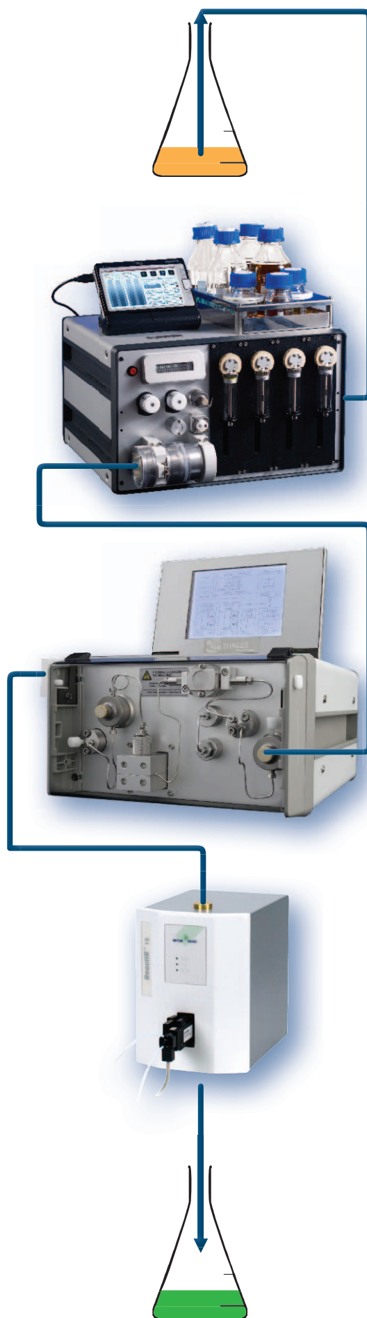
Figure 1. Tandem Continuous Flow Reactor and Analysis Setup
